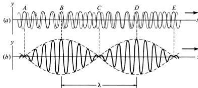
**(a): Two waves of slightly different frequencies,  $f_1$  and  $f_2$  add to form the resultant wave in (b)**
