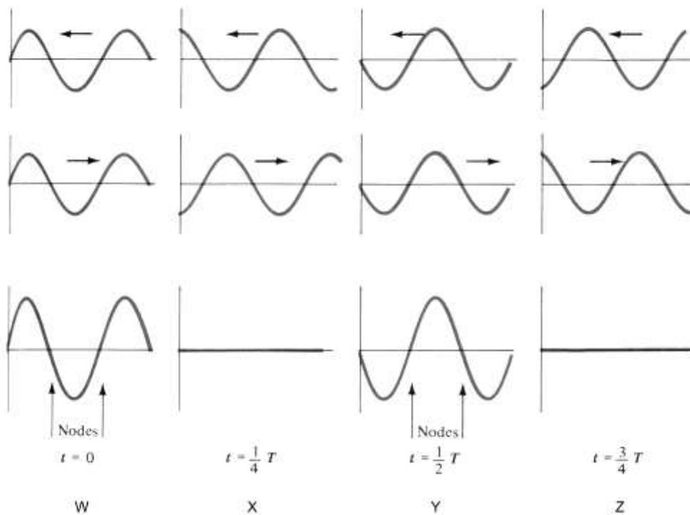
B. Waves on a “string” at time intervals of  $1/4T$ . [ 1.a. is a wave traveling to the left and 1.b. is a wave traveling to the right.] As they pass each other we have constructive interference occurring at W and Y and destructive interference occurring at X and Z. The shape of the string changes with time, but its displacement is always zero at the nodes.
