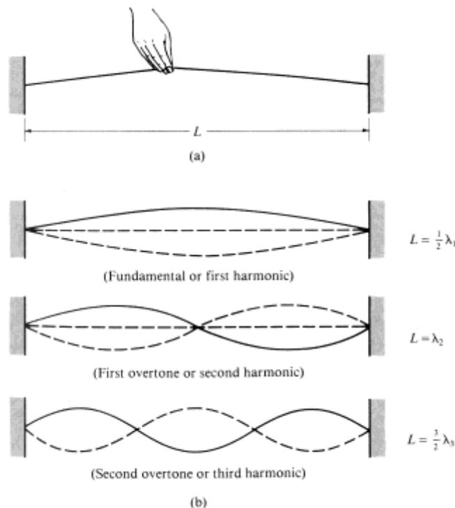
The lowest frequency that the string will vibrate to is called the fundamental frequency or one antinode or loop. Other resonant frequencies or natural frequencies are also called overtones and when they are integral multiples of the fundamental frequency they are also called harmonics.
