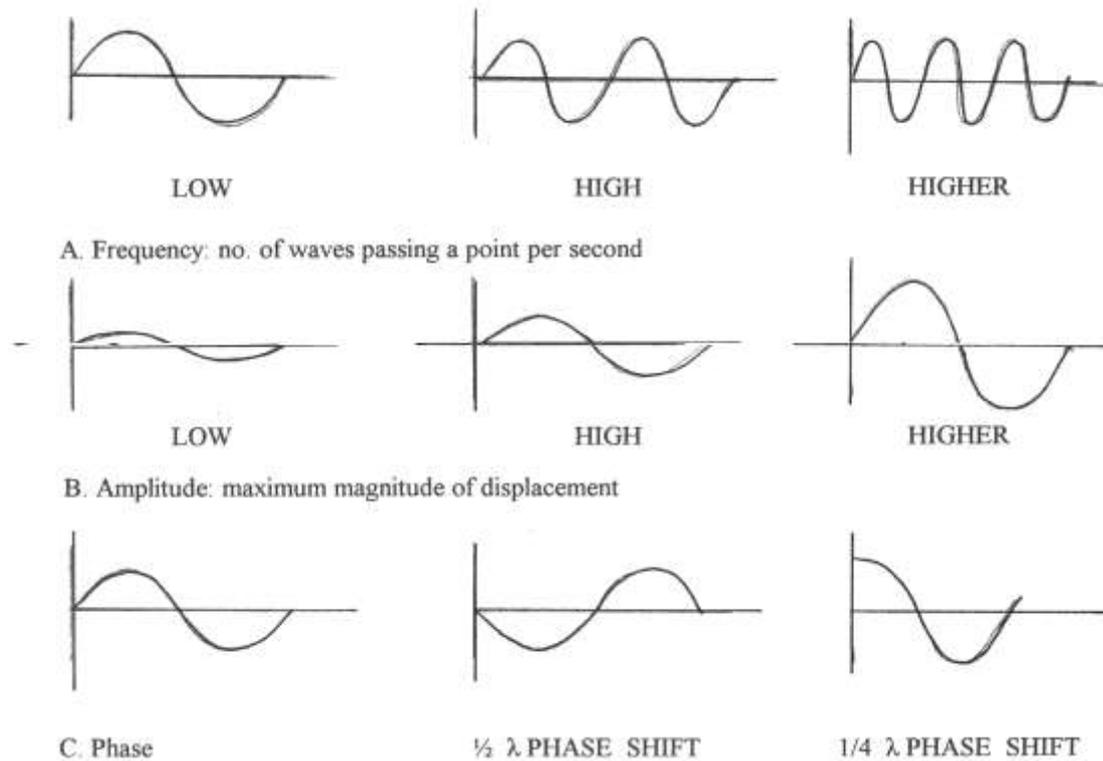
Electromagnetic waves require no medium in which to propagate. These waves are due to mutually induced time-varying electric and magnetic fields. When two or more waves travel, the resulting wave is the sum of the displacement associated with the individual waves. As shown in Chapter V we can view these changes as Constructive and Destructive Interference. Note Diagram 2.
